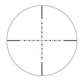
The crosshair has dots and dashes spread equally along the X and Y axis. The distance between two adjacent marks subtends to 1 milli-radian. The etched-glass reticle offers our discerning users the sharpest Mil-dot reticle for precise range estimation.
