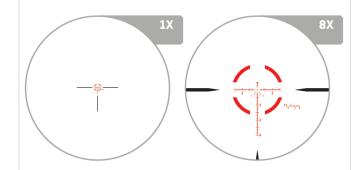
At 1X, a quick-to-acquire T-Dot enclosed within a 68 MOA segmented circle makes close up work, quick and to the point, functioning similarly to a dot sight. At higher magnifications the reticle opens up to provide users with a crisp 1 MOA center dot, range estimation out to 600 yards, and hash marks up to 60 MOA vertically for holdover and 30 MOA horizontally left and right in 2 MOA increments.
