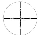
The crosshair has multiple dots spread equally along the X and Y axis. The distance between two adjacent marks subtends to 1 milli-radian. The traditional wire reticle is robust and holds up against strong recoil and offers a clear aiming reference without compromise.
