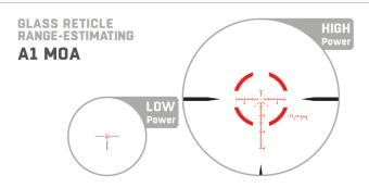
At 1X, a quick-to-acquire T-Dot enclosed within a 68 MOA segmented circle makes close up work, quick and to the point, functioning similarly to a dot sight. At higher magnifications the reticle opens up to provide users with a crisp 1 MOA center dot, range estimation out to 600 yards, and hash marks up to 60 MOA vertically for holdover and 30 MOA horizontally left and right in 2 MOA increments.
